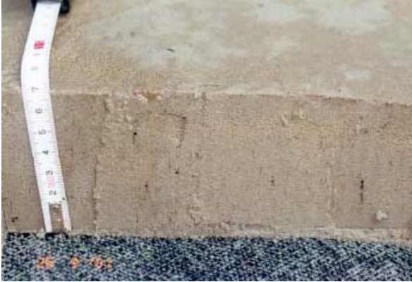
Photograph 1. Check of layer thickness after excavation
