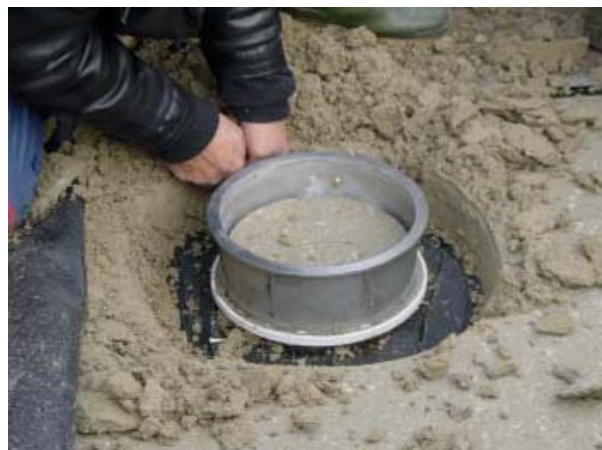
Photograph 4. Sample ring developed for the excavations
