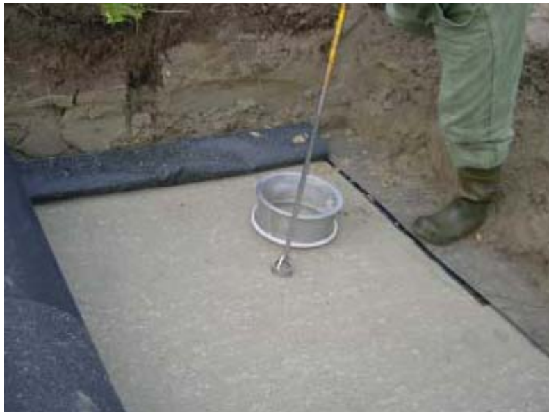
Photograph 3. Taking a sample during excavation
